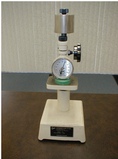
Durometer gauge with conveloader stand. The conveloader helps to make the durometer readings more consistent by controlling the force and rate which is applied to the gauge as well as keeping it perpendicular to the sample being tested.
